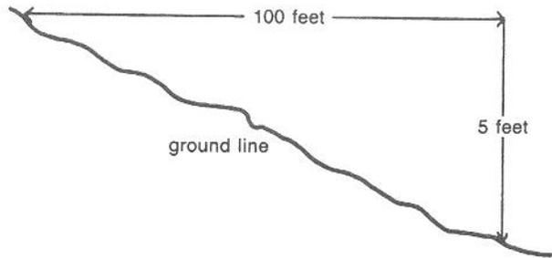
**Figure 8. Diagram showing a 5 percent slope**
